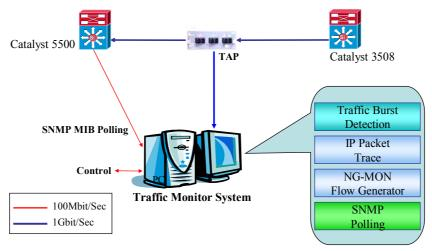
Figure 1: Overview of Traffic Monitoring Modules
