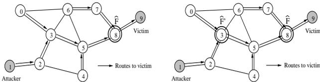
**Figure 2: Left: With route-based filtering executed at node 8, the spoofable address range at attack site 1 is reduced from  $S_{1,9} = \{0, 1, 2, 3, 4, 5, 6, 7, 8\}$  to  $\{0, 1, 2, 3, 4, 5\}$ . Right: Distributed filtering with filter  $\hat{F}$  at AS 3, the spoofable range further reduces to  $S_{1,9} = \{1, 2\}$ .**
