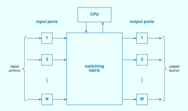
• Any input port can send to any output port
