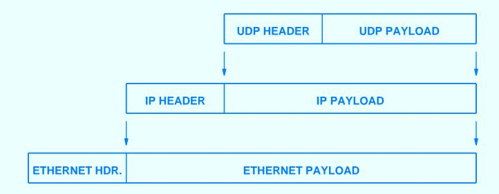
• Field in each header specifies type of encapsulated packet
