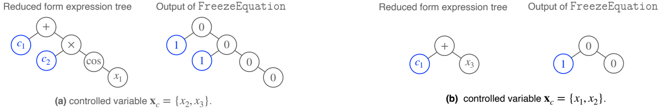
Figure 7: Visualization of the FreezeEquation function. 0 implies the node is non-editable and 1 implies the node is editable, by the GP algorithm. The FreezeEquation function will increase the probability of finding expression trees with close-to-zero fitness scores.
