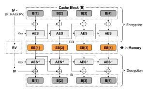
Figure 4. Encryption mechanism that directly encrypts cache blocks with AES.
