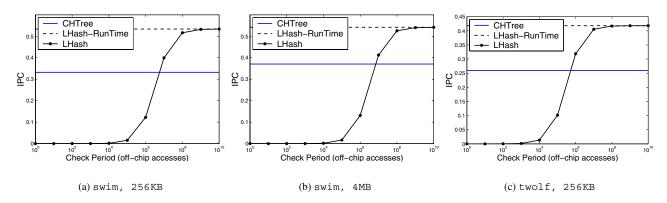
Figure 11. Performance comparison between LHash and CHTree for various checking periods. LHash-RunTime indicates the performance of the LHash scheme without checking overhead. Results are shown for caches with 64-B blocks. 32-bit time stamps and 128-bit hashes are used.
