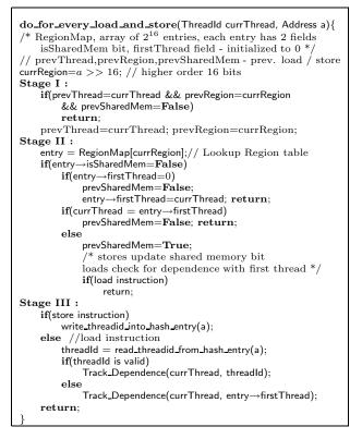
Figure 3: Pseudo-code for detecting shared memory dependences. The code shows the processing that is done for every memory load and store instruction. The 3 stages are clearly marked.
