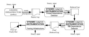
Figure 4: Implementation of our system showing each step of the framework.
