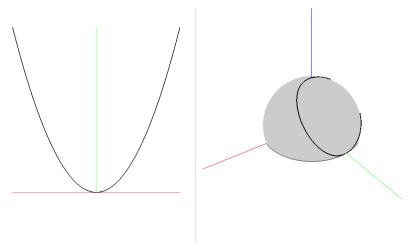
The parabola  $y = x^2$  homogenizes to  $yz - x^2 = 0$  with point at infinity (0,1,0) that converts the affine parabola into a loop.
