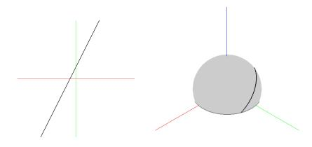
The line y = 2x + 2 homogenizes to 2x - y + 2z = 0 with point at infinity (1, 2, 0) that equals (0.447, 0.894, 0) in the hemisphere model. This point converts the affine line into a loop.
