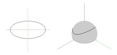
The ellipse  $x^2 + 4y^2 = 4$  homogenizes to  $x^2 + 4y^2 - 4z^2 = 0$  with no points at infinity, since the affine ellipse is already closed.
