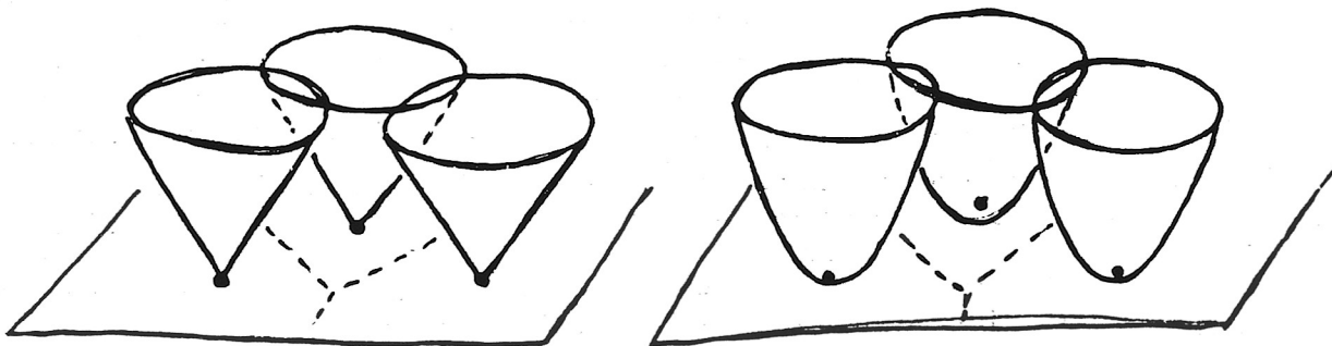
Figure 7.2: For each p \in S take a cone with apex p , vertical axis, and right opening angle. The lower envelope of the cones projects vertically to the Voronoi diagram of S . Similarly, we can take a paraboloid per point and project the lower envelope of the paraboloids.
