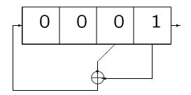
The bits that are shifted out the right side of the register are the key stream. They are XORed with the plaintext to form the ciphertext (or vice versa to decrypt).
