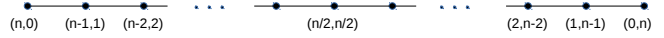
Figure 5. Privacy-constraint graph for K = 2 and general n . The vertices are labeled by the corresponding histogram. Two vertices are connected by an edge if their corresponding histograms are at an \mathbb{L}_1 -distance 2.
