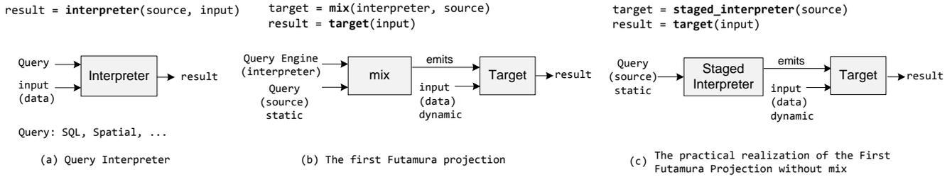
**Figure 2: Specializing query engines using the practical realization of the first Futamura Projection [64].**
