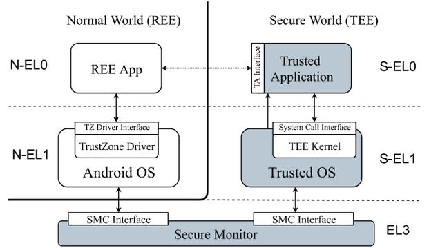
Figure 1. Software architecture of a TrustZone-assisted TEE system.
