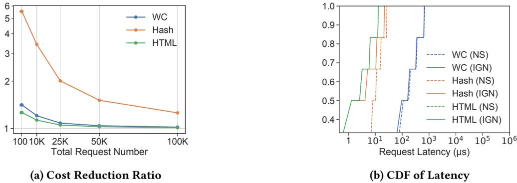
**Figure 5: Simulated improvement of using IGNITE (IGN) over a no-sharing (NS) approach in: a) cost (total CPU time), and b) request latency.**
