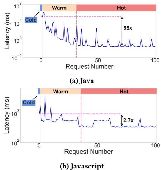
**Figure 1: Latency per request for a word count (Word-Count) workload on Java and Javascript runtimes for cold/warm/hot stages. These runtimes improve performance by 55x (Java) and 2.7x (JavaScript) through JIT compilation and code profiling. Periodic spikes occur due to garbage collection.**
