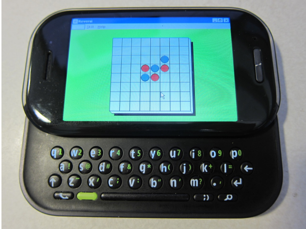
Figure 4. Experiment demonstrating an x86 Windows application (Reversi) on an ARM phone.
