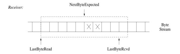
• sender, receiver maintain buffers MaxSendBuffer, MaxRcvBuffer
