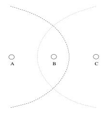
$\rightarrow$  two problems with using simple CSMA
