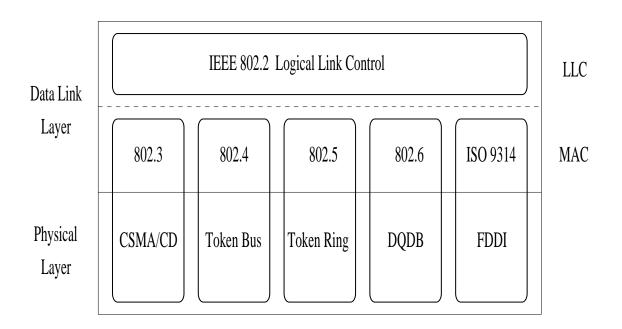
Logical link control: Isolation of common generic mechanisms including reliability and flow control.
