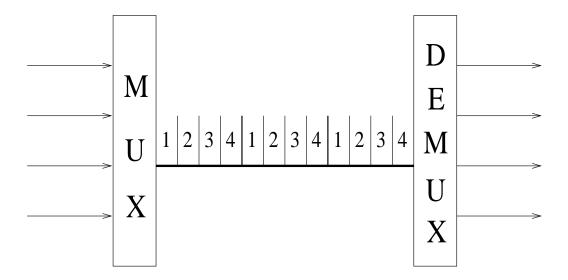
Clearly, bit rate of medium > data rate of signal; however, mostly used for digital transmission of digital or analog data (PCM, codec).
