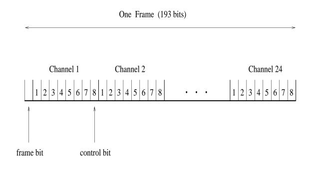
Assuming 4 kHz telephone channel bandwidth, Sampling Theorem dictates 8000 samples per second (125  $\mu$ sec/sample).
