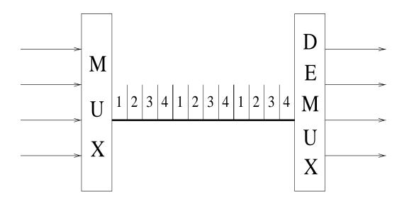
$\rightarrow$  router A: MUX (multiplexer, or combiner)  $\rightarrow$  router B: DEMUX (demultiplexer, or splitter)
