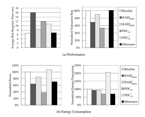
Figure 12: Performance and energy consumption comparison on an emulated storage system. The database transaction rate, power (energy/time), and energy consumption are normalized to the baseline. The energy consumption is evaluated for the specified number of transactions.
