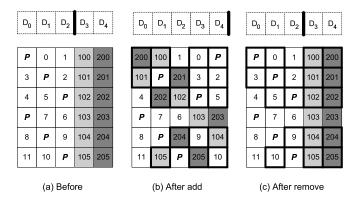
Figure 5: Randomized Shuffling. The graphics have the same meanings as in Figure 4. The transition from (a) to (b) shows the addition of disks  $D_3$  and  $D_4$  to a fast (hot) tier. The transition from (b) to (c) shows the result of moving those same disks into a slower (cooler) tier.
