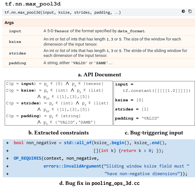
Figure 1: TensorFlow document helps our tool detect a bug that was fixed after we reported it to TensorFlow developers.
