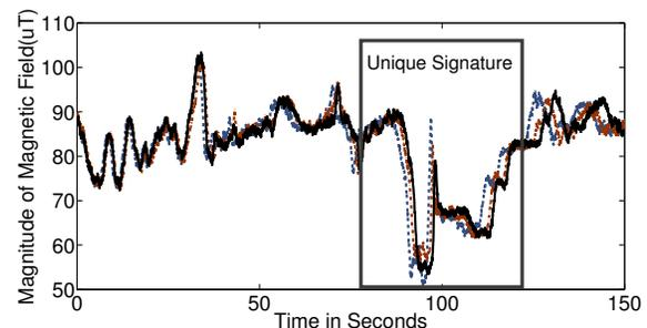
Figure 1: Magnetic signature near a networking lab.
