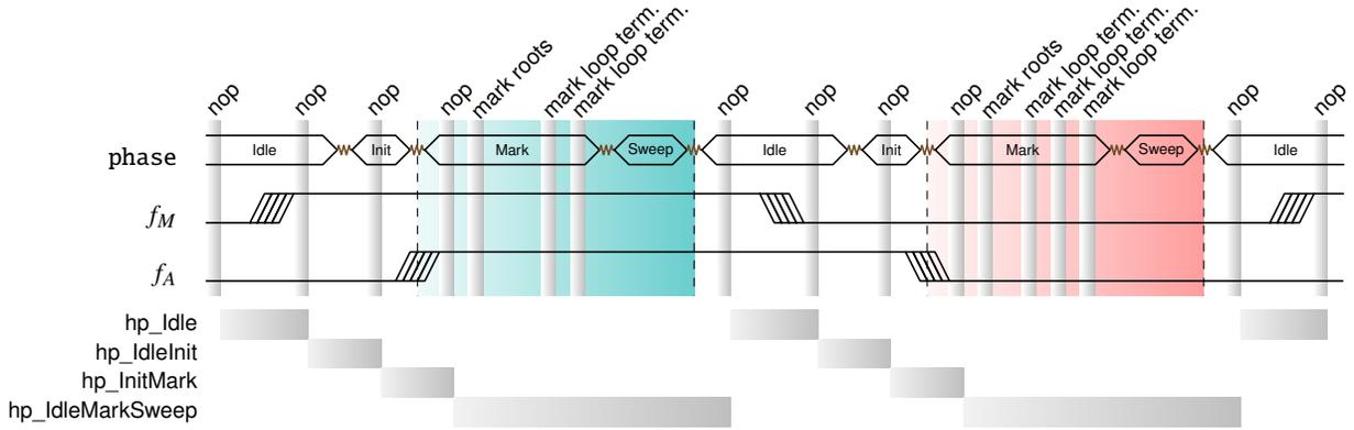
**Figure 3.** The mutators’ view of control state transitions and handshakes. The handshakes are annotated with their types at the top of the diagram. At the bottom is *handshake phase* that the mutator is in, which we discuss in §3.2.
