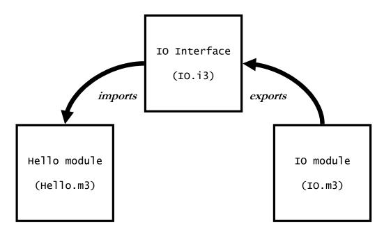
Figure 5. A Schematic of the IO Interface
