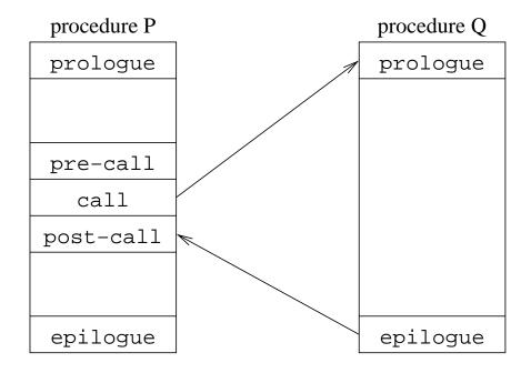
Each system has a standard linkage
