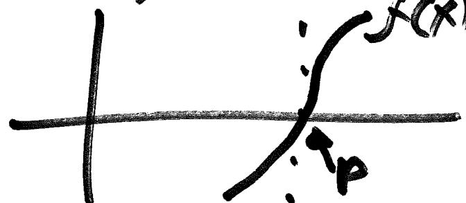
If the graph  $y=f(x)$  is shallow (close to horizontal) near  $(P, 0)$  then the root finding is "ill conditioned" i.e. the root finding may only have a few significant digits.
