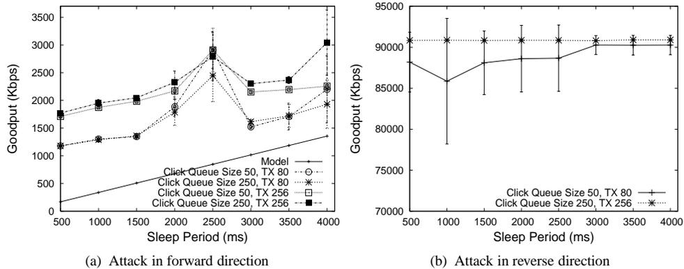
Fig. 8. Impact of varying the Click router queue and the transmit buffer ring of the network device driver on DETER. Attack packets are 64 bytes. The attack pulse length and RTT are set to 160 ms.
