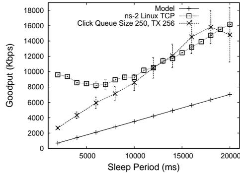
Fig. 9. Comparison of the average goodput from analysis, simulation, and Click (on DETER) for long sleep periods. Attack packets are 64 bytes. Queue size in ns-2 and output device buffer ring in Click is 256. The attack pulse length and RTT are set to 160 ms.
