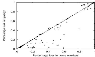
Fig. 4. Average packet loss for 660 network paths in home overlays and Synergy, where half of the paths are in home overlays and the other half is in Synergy. In the figure, 112 points exceed 0.3 for Synergy (horizontal line) while 128 points exceed 0.3 for home overlays (vertical line). In addition, 89 points exceed 0.5 for Synergy, but 105 points exceed 0.5 for home overlays.
