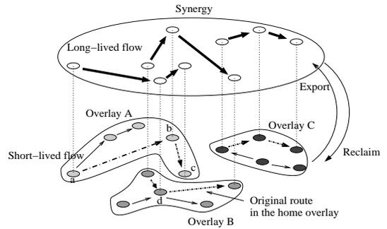
Fig. 1. Overlay internetworking architecture: An overlay internetwork is constructed among exported hosts. Long-lived flows (dash-dot lines) in home overlays are replaced by Synergy routes (thick lines) if this will improve performance.
