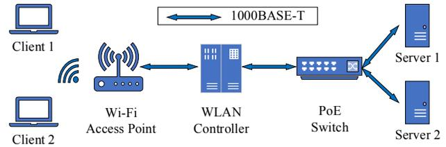
Figure 1: Experimental testbed
