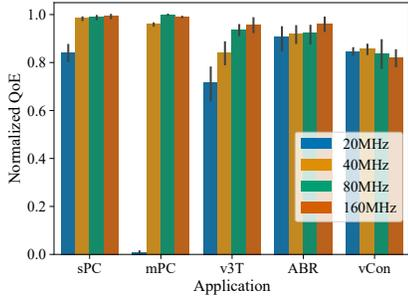
Figure 5: QoE for different channel widths.
