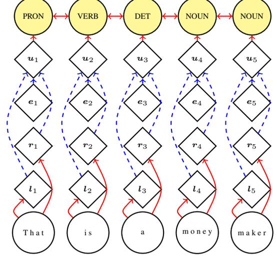
Figure 2: A demonstration of the neural CRF encoder.  $l_t$  and  $r_t$  are the output of the forward and backward character-level LSTM of the word at position  $t$  in a sentence, and  $e_t$  is the word-level embedding of that word.  $\mathbf{u}_t$  is the concatenation of  $e_t$ ,  $l_t$  and  $r_t$ , denoted by blue dashed arrows.
