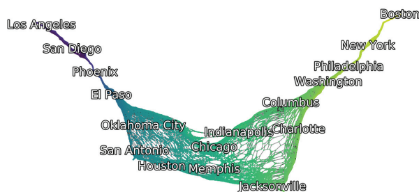
Fig. 18 A spectral embedding of the US Highway Network corresponding to the first and second nontrivial eigenvectors of the Laplacian matrix. The embedded locations of major cities are labeled as well. Node color is determined by the true longitude of a node, which shows that the first eigenvector of the Laplacian correlates with an east-west split of the network. This global embedding, however, compresses major regions of the northeastern US (Washington, New York, Boston) as well as the western US (Los Angeles, San Diego, Phoenix).
