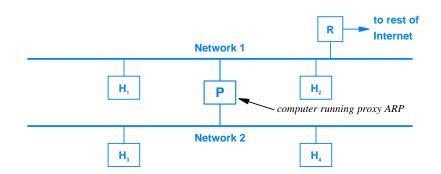
Figure 6.5 Illustration of two networks using proxy ARP.
