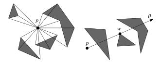
If p and w bound the same obstacle, w is visible from p if pw is disjoint from the interior of the obstacle.
