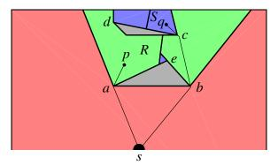
A shortest path map (SPM) for a point s and disjoint polygonal obstacles O is a planar subdivision where all the points in a face have the same sequence of O vertices on their shortest paths to s.
