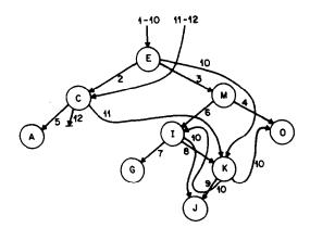
Insertion of E at time 1, C at time 2, M at time 3, 0, A, I, G, K, and J then deletion of M at time 10, E at time 11, and A at time 12. Pointers are labeled with their time stamps.
