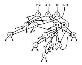
Insertion of E, C, M, 0, A, I, G, K, and J at times 1-9 then deletion of M, E, and A at times 10-12.
