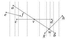
► The vertical order is computed at the left endpoint a of an edge ab with respect to an edge ef with e<sub>x</sub> ≤ a<sub>x</sub> < f<sub>x</sub>.
