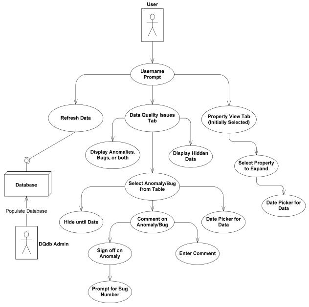
We decided to feature the Use Case Diagram before the UI Flow Model in order to get the reader acquainted with the simple ideas of the GUI design. The only item of note in this diagram is that the Database is actively being populated by another agent. In order to explain this diagram, we provided some use cases relevant to the above use case diagram.
