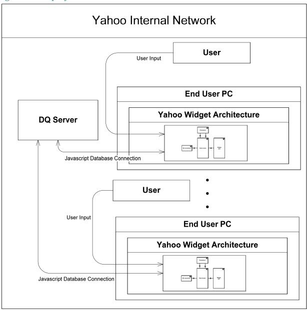
This diagram is pretty straightforward. We feature the diagram sitting inside the yahoo network with each end user pc containing the necessary architecture to run the widget that we are developing. Each widget that is running will have a connection to the DQ server through the JavaScript COM model and there can potentially be many connections to the database as there will be multiple deployments of our software.
