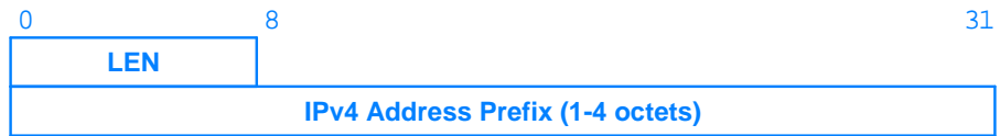
Figure 13.7 The compressed format BGP uses to store an IPv4 destination address and the associated address mask.
