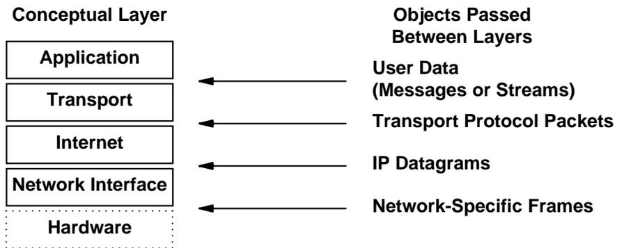
**Figure 3.1** The conceptual organization of TCP/IP protocol software into layers.
