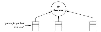
**Figure 2.2** Communication between the network device drivers and the process that implements IP uses a set of queues. When a datagram arrives, the network input process enqueues it and sends a message to the IP process.
