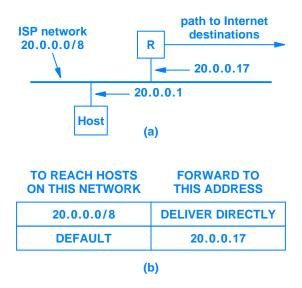
**Figure 8.3** (a) An example Internet connection using IPv4 addresses, and (b) the forwarding table used in the host.
