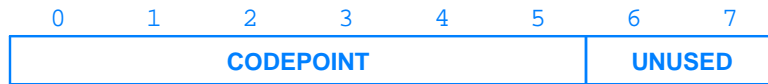
Figure 7.7 The differentiated services (DiffServ) interpretation of bits in the IPv4 SERVICE TYPE and IPv6 TRAFFIC CLASS header fields.
