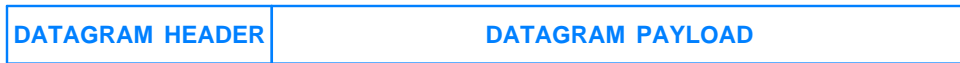
Figure 7.2 General form of an IP datagram, the Internet analogy of a network frame.
