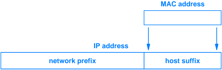
Figure 6.1 An illustration of a direct mapping scheme in which a computer's hardware address is embedded in the computer's IP address.
