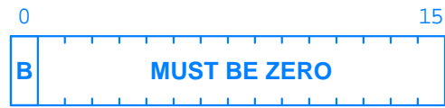
Figure 22.2 The format of the 16-bit FLAGS field in a DHCP message. The leftmost bit is interpreted as a broadcast request; all others bits must be set to zero.
