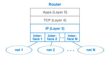
Figure 17.1 The protocol stack in a traditional router with layers involved in forwarding a transit datagram highlighted.
