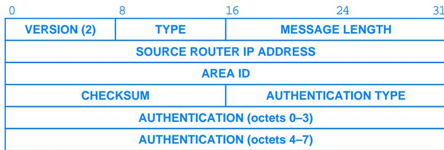
**Figure 14.9** The fixed 24-octet OSPFv2 header that appears in each message.
