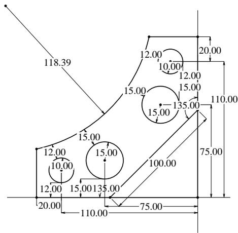
Figure 6: Solution 4 of the L(CC,CC) problem of example 3
