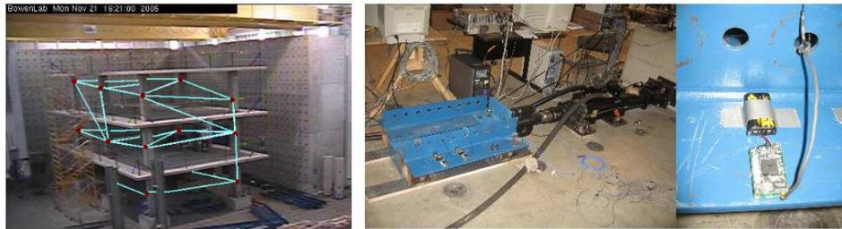
**Figure 1.9** Operational tests – electrohydraulic rams excite the structure and response is measured through a variety of self-organizing sensors.
