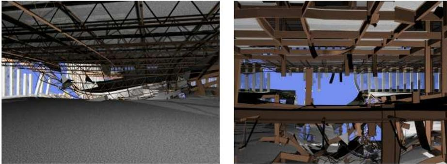
**Figure 1.6** Damage to Floors 95 and 96 (left); reverse angle shot from floor 96 (right). Note the detailed geometry of the spandrel beams and core beams represented by line elements in the simulation.
