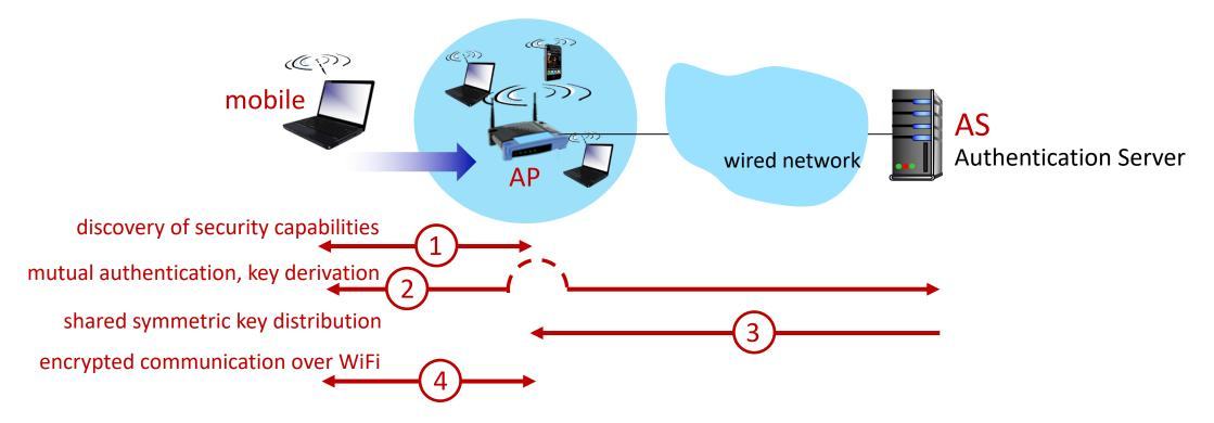
) encrypted communication between mobile and remote host via AP
