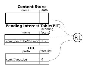
Figure 2: Components of NDN router
