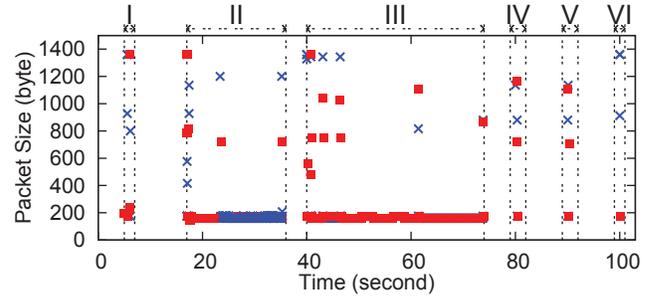
Fig. 3. The IPSec packets of six Wi-Fi calling events over time (×: uplink packets; ■: downlink packets; I/VI: Activating/Deactivating Wi-Fi calling; II/III: Receiving/Dialing a call; IV/V: Sending/Receiving a text).
